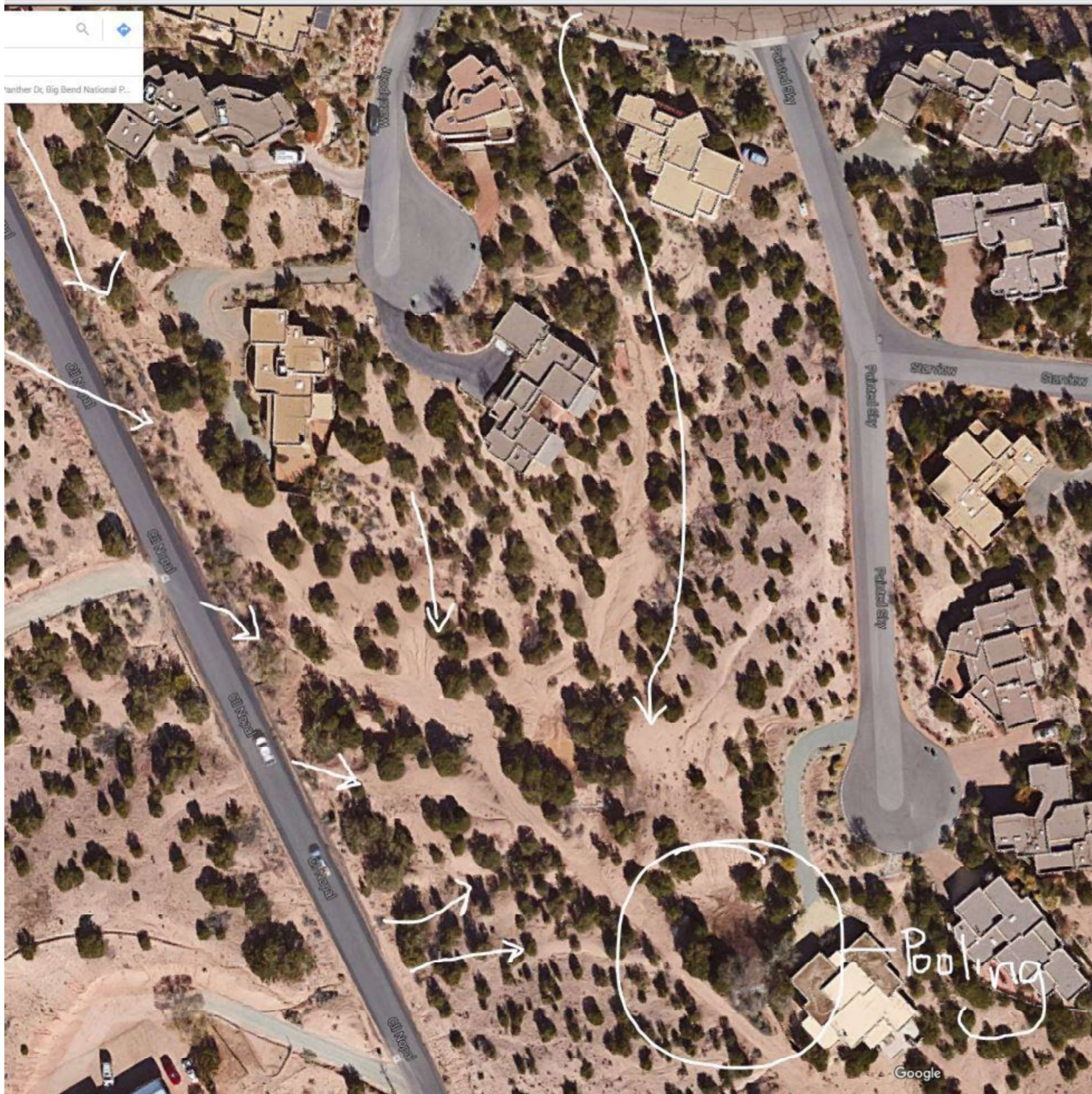
Aerial map of Arroyo Nopal describing the direction of water flow, catch basin locations and road locations. 2016
